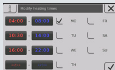
Fig. 2 View of the heating times (individually adjustable)
