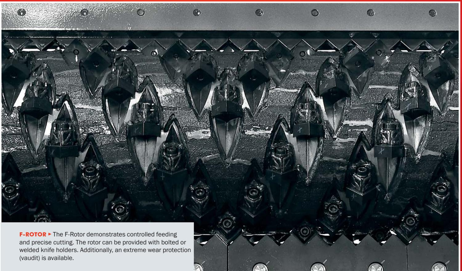
**F-ROTOR** ▶ The F-Rotor demonstrates controlled feeding and precise cutting. The rotor can be provided with bolted or welded knife holders. Additionally, an extreme wear protection (vaudit) is available.
